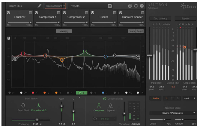
Neutron's processors include an EQ, compressor, transient shaper, exciter and limiter.
